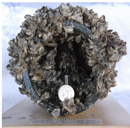
Quagga mussel infested pipe. Photo from Idaho Agriculture. www.agri.state.id.us
